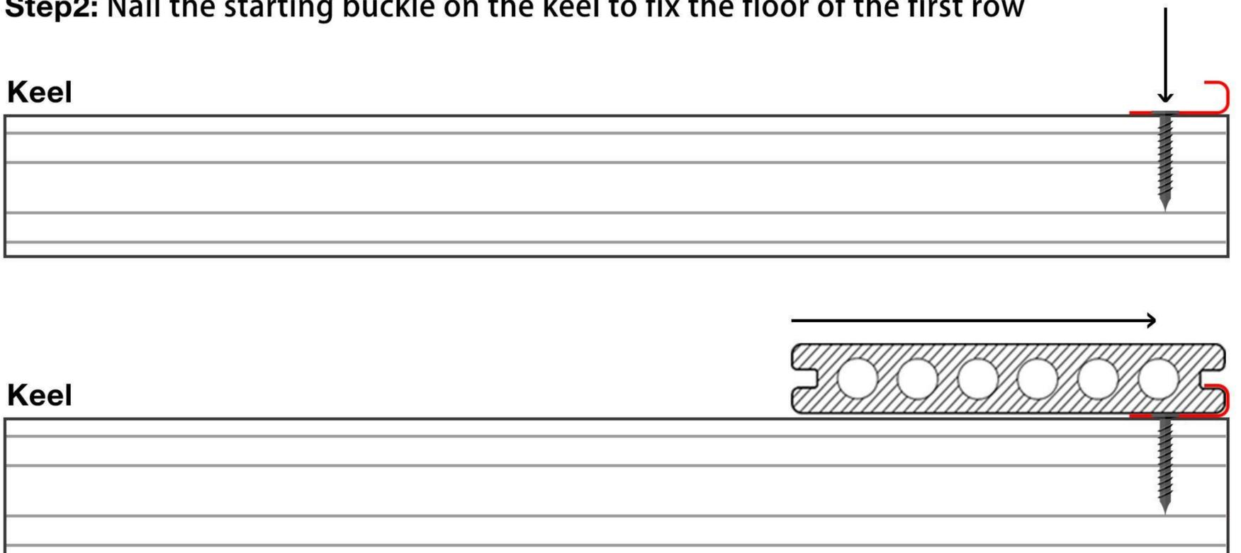
**Step3:** Install the fasteners between the floors and secure the second row of floors
