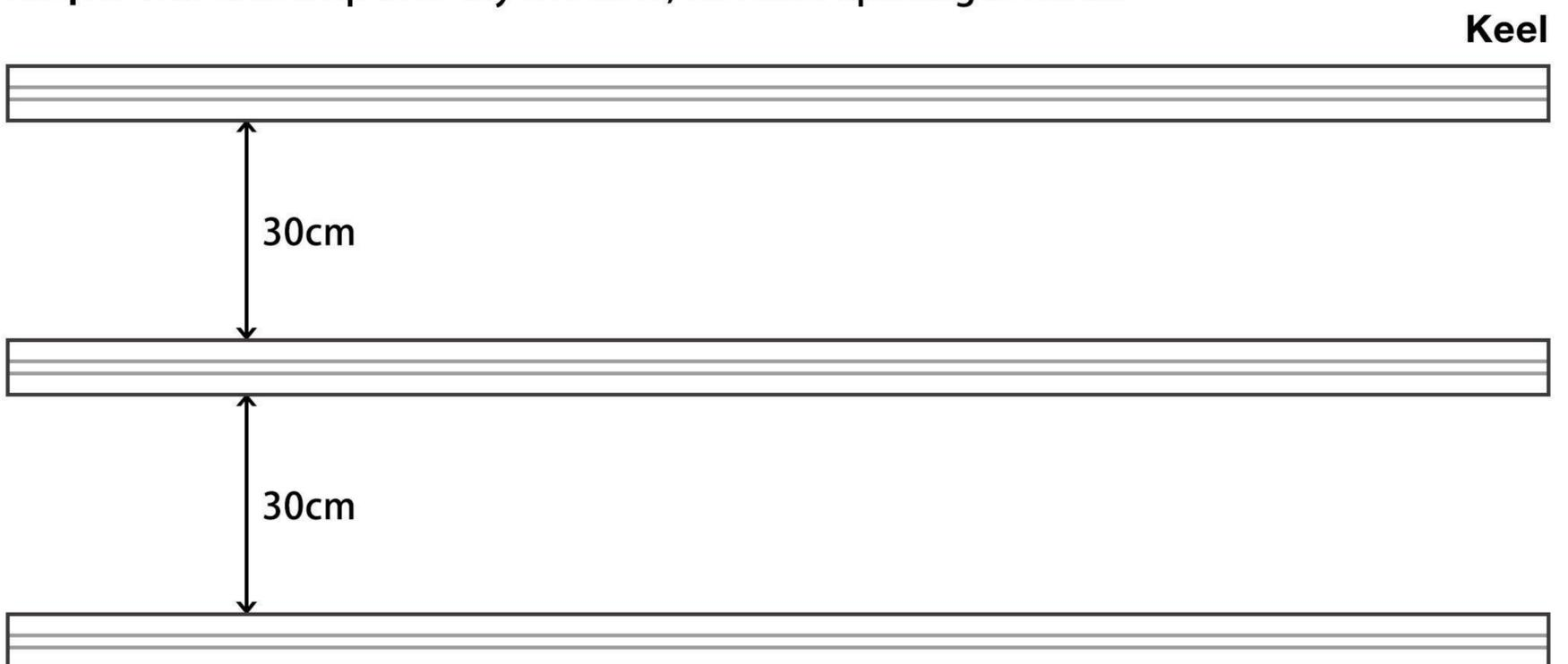
**Step2:** Nail the starting buckle on the keel to fix the floor of the first row
