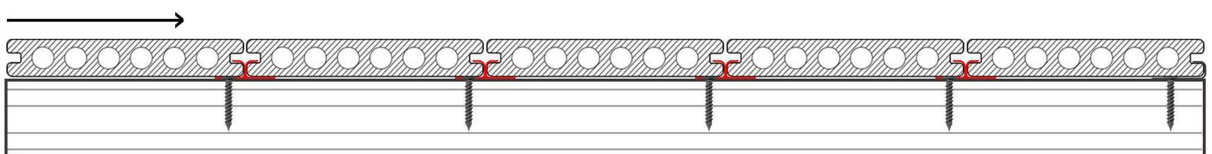
**Step5:** Screw the screw into the last wooden board and complete the installation
